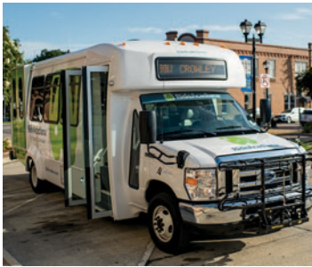
Two 16-seat, ADA-compliant vehicles, equipped with a lift, secure area for two wheelchairs, and bike rack
